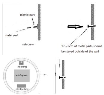
Hange up the mirror on screw and make sure stable. testing Mirror working
